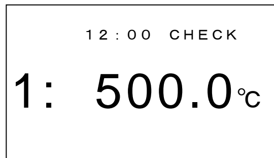
< One-selected-channel extended display screen during check measurement >
